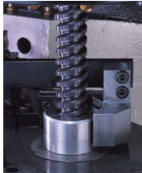
MQL Broaching Realize a small amount of coolant broaching by turning cutting oil into mist.
