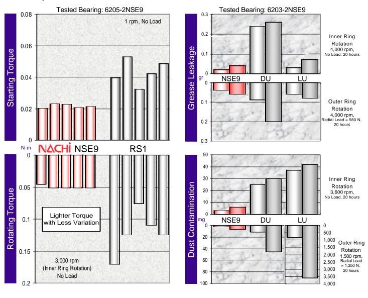
With **NACHI NSE9** Sealed Bearings, **more than 20W of energy can be saved** per bearing at 3,000 rpm.
